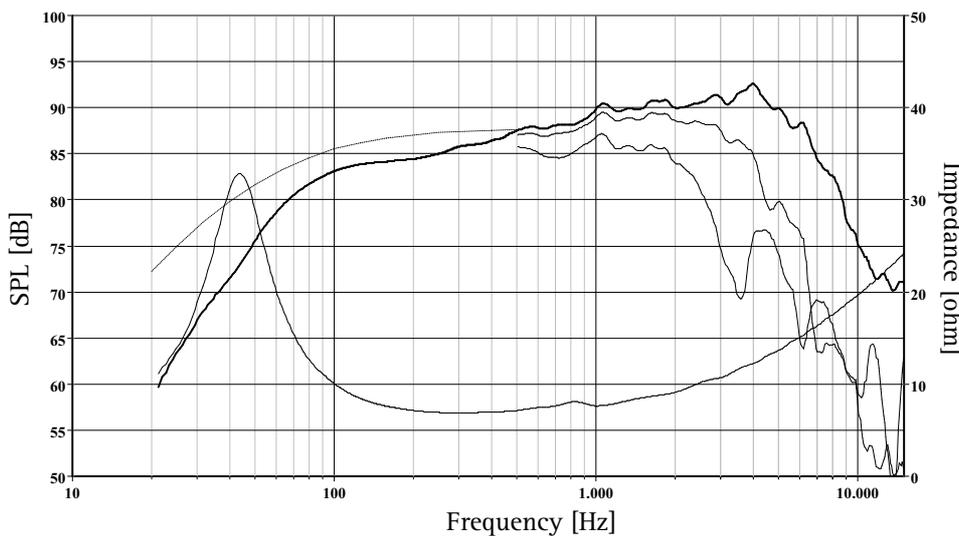
The frequency responses above show measured free field sound pressure in 0, 30, and 60 degrees angle using a 10L closed box. Input 2.83 V<sub>RMS</sub>, microphone distance 0.5m, normalized to SPL 1m. The dotted line is a calculated response in infinite baffle based on the parameters given for this specific driver. The impedance is measured in free air without baffle using a 2V sine signal.
