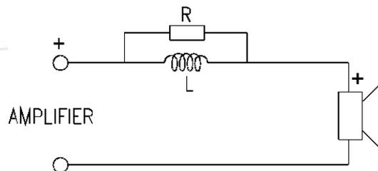
Please see the effect of two proposed networks on the axial sound pressure frequency response measured in a 60 litre closed cabinet. Black: No network. Red: 0.82mH and 6.8 Ohms. Blue: 1.5mH and 15 Ohms. The parallel resistor controls the high frequency attenuation. A larger resistance results in more attenuation. Metal film resistors of at least 5 Watts are recommended. Please make sure that the inductor is wound from a heavy conductor for a low series resistance, preferably less than 0.5 Ohms.
