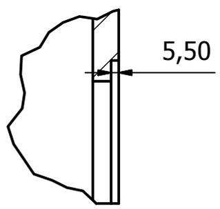
This component must be clean and with a surface energy not less than 40 mN/m (dyn/cm).
